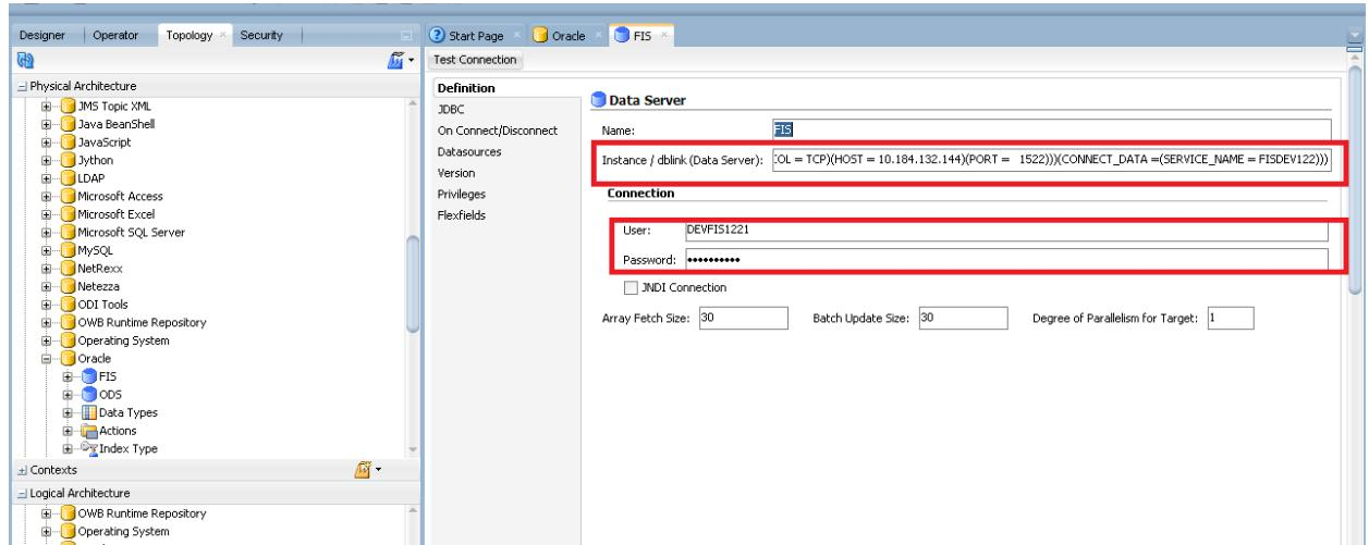
Then go to the JDBC and update the driver details of the source schema and test the connection
